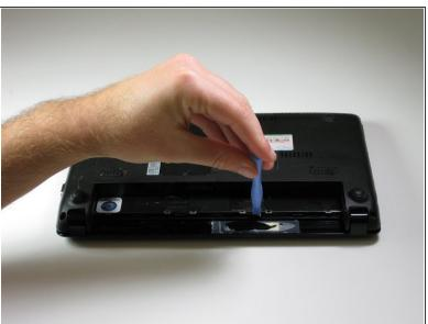
Use a plastic opening tool to pull up the four metal latches in the battery cavity that is located on the bottom of the laptop.
