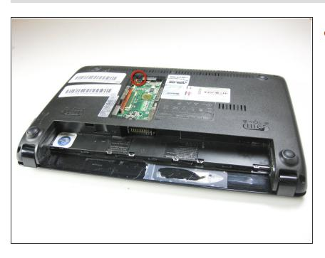
Remove the single 6.65 mm screw next to the RAM socket.
