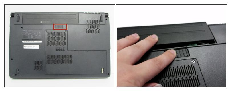
• While holding down the slider, gently remove the battery.
