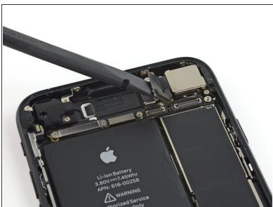
Use the flat end of a spudger to disconnect the rear-facing camera connector.
