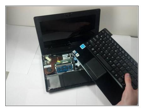
The keyboard is now fully disconnected and can now be removed from the main body of the Asus Eee PC 1018P.
