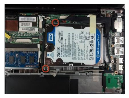
Use a Phillips #0 screwdriver to remove the two 4.52 mm screws securing the hard drive case to the laptop.
