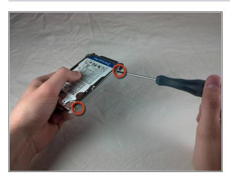
Use a Phillips #0 screwdriver to remove the four 3.68 mm screws securing the hard drive case to the hard drive. There are two on each side of the hard drive case.
