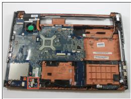
Disconnect the white cable near the bottom of the laptop.
