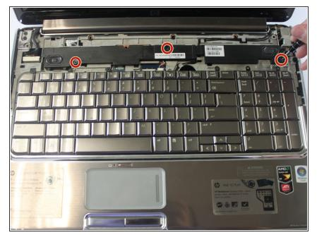
Remove the three Phillips PM2.5×3.0 screws, located on the speaker, with a Phillips #00 screwdriver.
