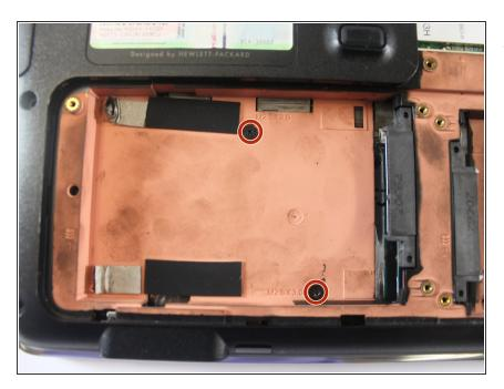
Remove the two Phillips PM2.5×4.0 broadhead screws with a Phillips #00 screwdriver.
