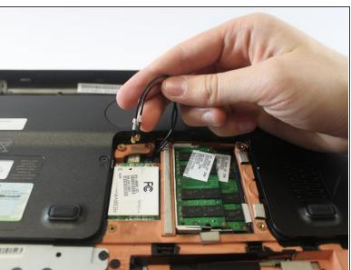
Disconnect the WLAN antenna cables.
