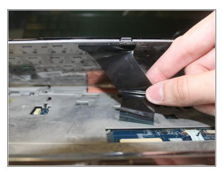
Disconnect the black zero insertion force connector in order to completely remove the keyboard.
