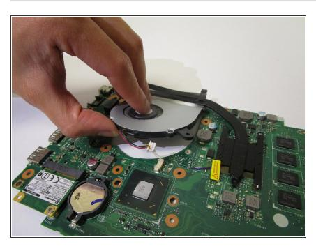
Lift the fan off to remove it from the motherboard.
