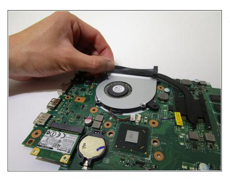
Detach the tape that connects the fan to the heatsink.
