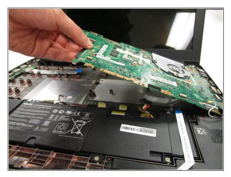
Gently lift the motherboard out of the casing.
