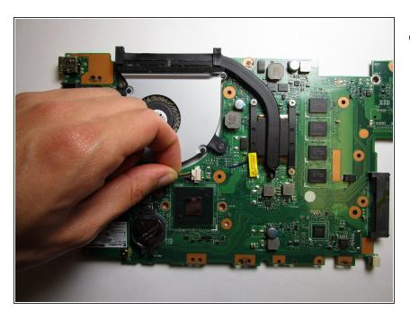
Disconnect the fan from the motherboard by pulling the power cable connector.
