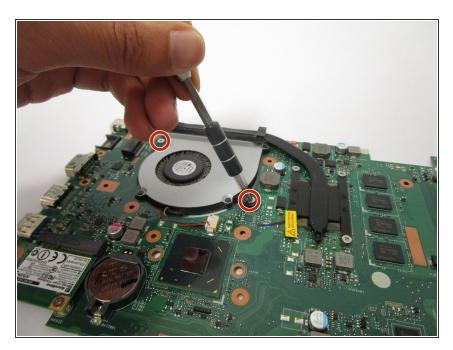
Remove the two 5.5mm screws using a Phillips #0 head screwdriver.
