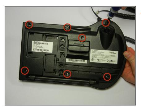
Remove the seven 8mm Phillips #2 screws.
