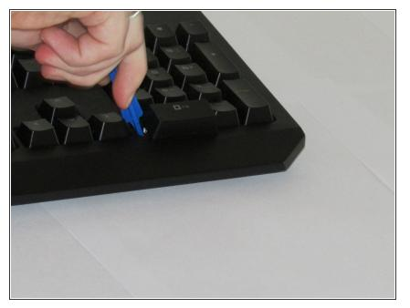
If the problematic key is still attached, place the edge of the medium blue pry tool under the key. Then gently pry up until key is detached.
