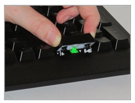
Some larger keys may also be held in by two small metal hooks. To separate them gently slide the key left to separate right hook, then to the right to separate the left hook.
