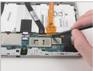
Use the flat end of a nylon spudger to pry up the **brown** plastic tab securing the orange ribbon cable.
