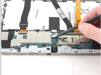
Use the pointed end of a nylon spudger to pry the two battery connections away from the motherboard.
