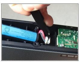
Locate the battery connection and unplug it using a pair of metal tweezers.
