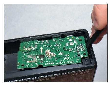
Remove the I/O board from the rest of the speaker. A plastic spudger can aid in this process if it is inserted into the edge as shown and gently pried.
