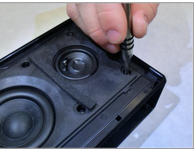
Locate the eight 8.9 mm screws on the face of the speaker assembly and remove them using a Phillips head #2 screwdriver.
