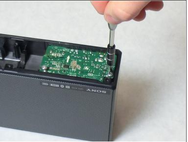
Locate the remaining two 3.5 mm screws on the bottom of the I/O board and remove them using a Phillips head #2 screwdriver.
