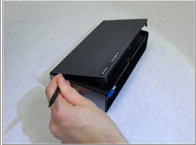
Insert a plastic spudger into the seam where the forward facing metal speaker cover meets the speaker body and gently pry it upward until it releases.
