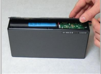
Insert a plastic spudger into the seam on the bottom panel and lift it away from the rest of the speaker.
