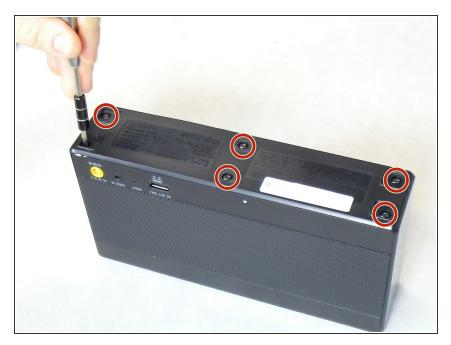
Locate the six 9 mm screws on the bottom of the speaker and remove them using Phillips head #2.
