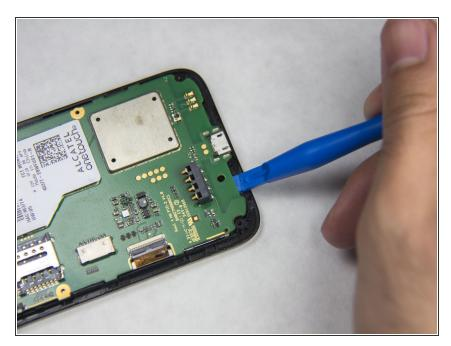
Insert one of the plastic opening tools into any side of the main circuit board and gently pry it loose from the front cover. Repeat the process all around the circuit board.
