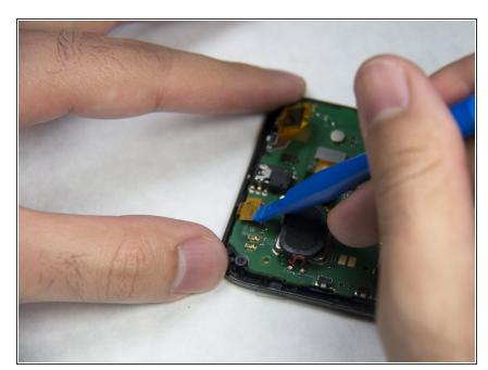
Use a plastic opening tool to lift the front camera press-fit connector free.
