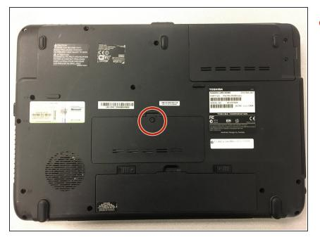
• Remove the Phillips #0 7-mm screw from the back of the computer.
