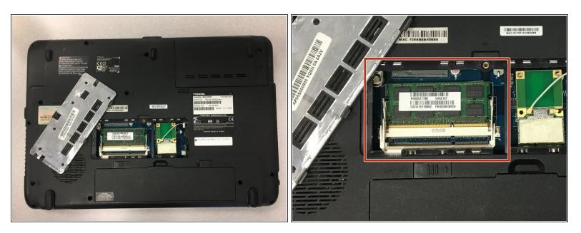
Remove the plate to access the RAM stick.
