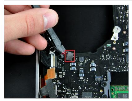
Use the flat end of a spudger to pry the subwoofer cable connector straight up off the logic board.
