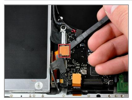
Use the flat end of a spudger to pry the optical drive cable connector straight up off the logic board.
