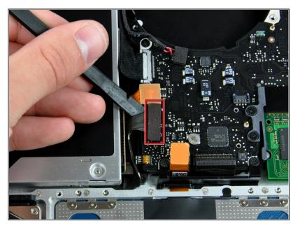
Use the flat end of a spudger to pry the hard drive cable connector straight up off the logic board.
