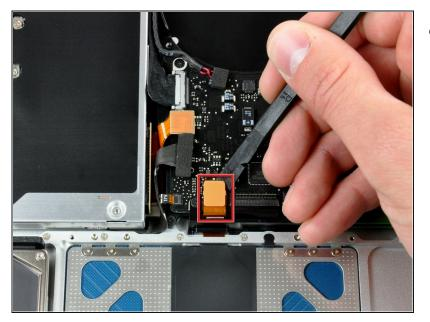
Use the flat end of a spudger to pry the trackpad connector straight up off the logic board.
