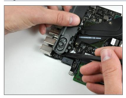
Use the flat end of a spudger to separate the left speaker assembly from the adhesive securing it to the logic board.
