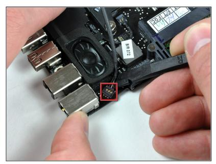
Use the flat end of a spudger to pry the microphone cable connector up off the logic board.
