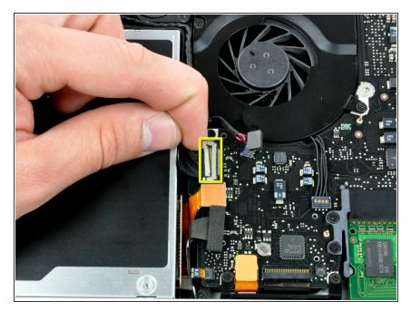
Disconnect the camera cable by pulling the male end straight away from its socket.
