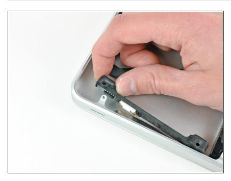
Pull the front hard drive bracket containing the IR sensor/sleep LED away from the front edge of the upper case.
