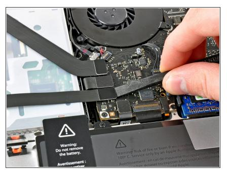
• Use the flat end of a spudger to pry the hard drive cable connector up from its socket on the logic board.
