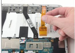
• Remove all three ribbon cables by gently pulling the cables away from the ZIF connectors.
