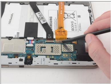
Use the flat end of a nylon spudger to pry up the **brown** plastic tab securing the orange ribbon cable.
