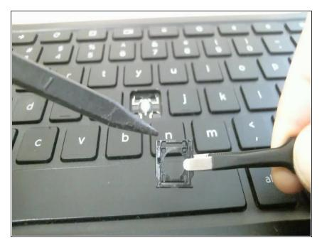
Line up the 2 outer corners and the bottom inner corners of the plastic bracket with the 4 metal clips connected to the palmrest.
