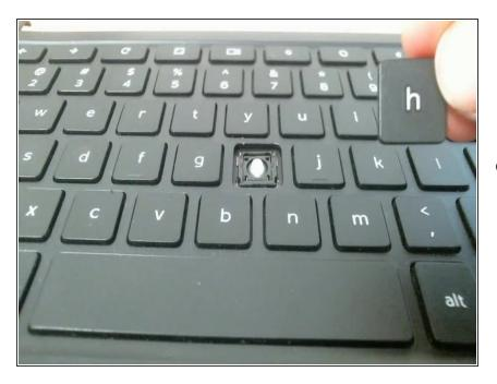
Place the key on top of the plastic bracket and press down. If the plastic bracket is on correctly and
