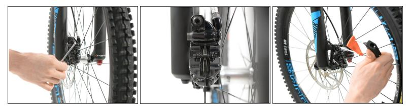
• The adjustment procedure for the front brake is the same as for the rear brake. Loosen the two screw nuts, position the brake so that the brake disc doesn't roam to one side of the brake caliper, tighten screw nuts afterwards with 9-10 Nm.
