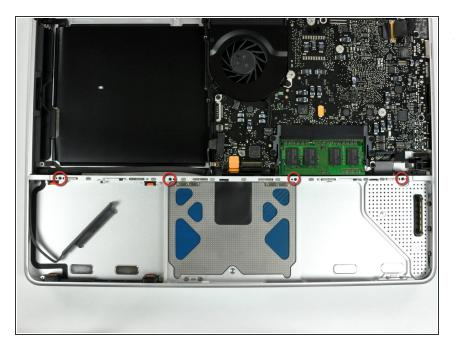
Remove the four 10.3 mm Phillips screws securing the mid wall to the upper case.
