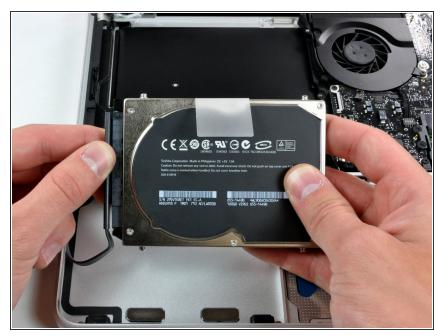
• Lift the hard drive out of its supports and disconnect the SATA cable by pulling the connector straight away from the hard drive.
