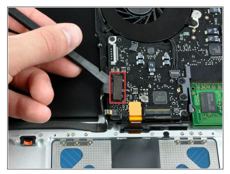
• Use a spudger to pry the hard drive cable connector straight up off the logic board.
