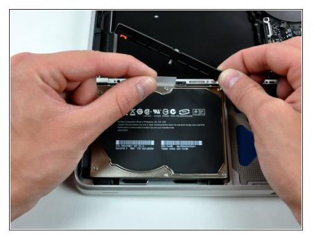
Lift the hard drive by its plastic pull tab and remove the freed hard drive bracket.
