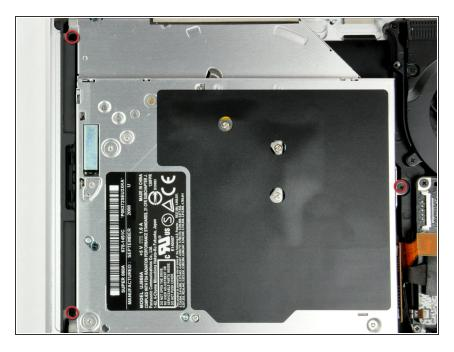
Remove the three 2.5 mm Phillips screws securing the optical drive to the upper case.
