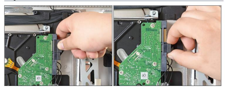
• Disconnect the SATA power and data cables from the hard drive by pulling them straight away from the hard drive.
