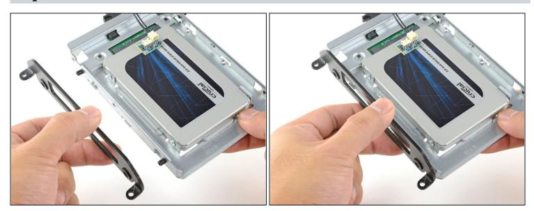
• Attach any mounting brackets removed from the old hard drive onto the enclosure.
