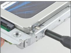
Use a Phillips screwdriver to install the four silver screws (two on each side) along the edges of the SSD to secure it to the enclosure.
