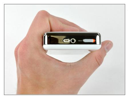
i Before opening your iPod, ensure that the hold switch is in the locked position. The orange bar should be visible, indicating hold is active.
