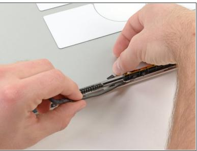
Carefully pull the display data cable through the recess located near the left hinge.
