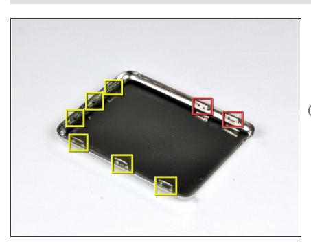
The rear panel is secured to the front case by eight clips permanently attached to the rear
