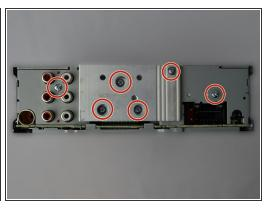
• Use the Phillips #0 Screwdriver to remove the screws off of the metal case.
