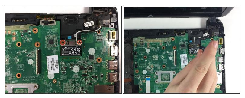
Remove the two 4.0 mm screws using a Philips #00 head screwdriver.
