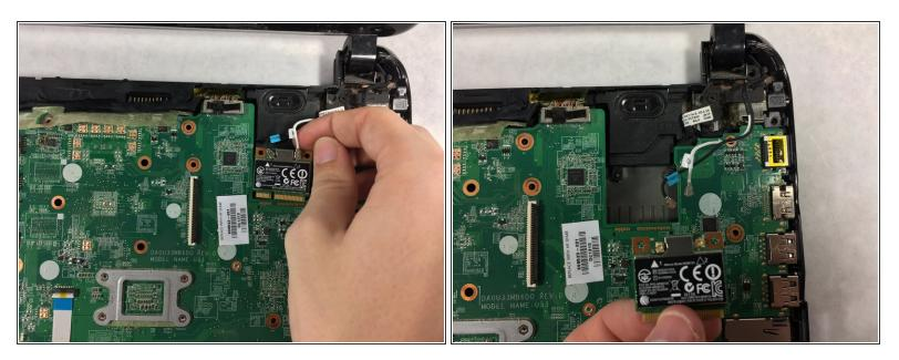
• Slide the card upwards and outwards to detach it from the motherboard.
