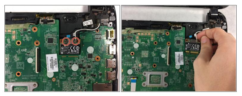
• Detach the two wires connecting to the motherboard to the wireless card.
