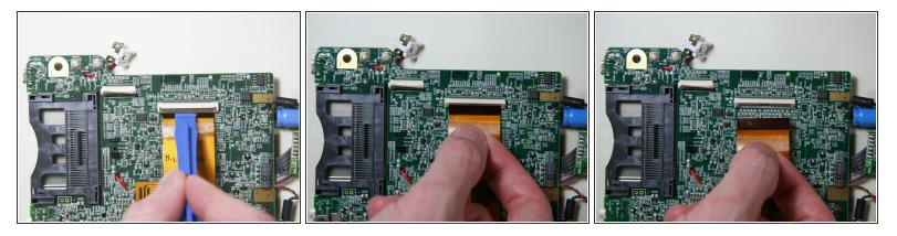
• Open the display connector by lifting on the brown latch with a plastic opening tool or a finger until it is in a vertical position.
