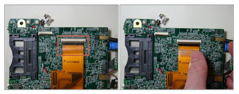
• Peel back the tape on the display ribbon cable connector.
