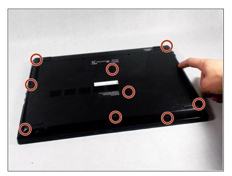
Unscrew the 10 9.0 mm screws holding the back panel on using a Phillips head #1 screwdriver.
