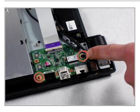
Remove the two 5.0 mm screws, using a Phillips #1 screwdriver, once the cable is out of the way.
