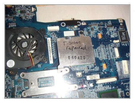
The new alloy shim is under the existing thin shim. I've done more than 20 of these repairs & had 100% success rate I always do the same to the CPU (might as well your already in there).,
