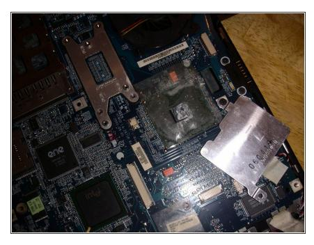
this is the culprit, as you can see the shim can easily overheat & go concave lifting off the chip.
