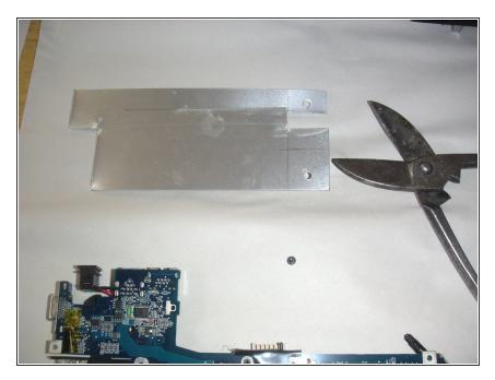
cut a thin piece of alloy to the same size as the existing shim, i used an old alloy door push plate(easy to cut) & is the ideal thickness
