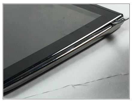
• Flip the tablet so the screen is facing upward, and use the metal spudger to pry apart the screen from the side pieces.
