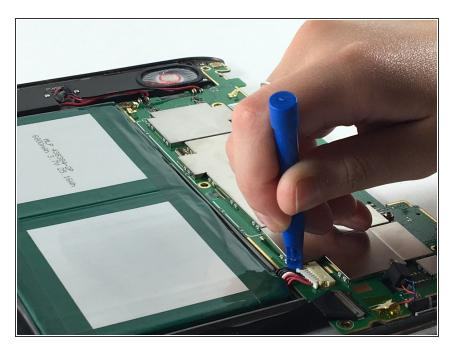
• Use the plastic opening tool to push out the wires connecting the battery to the motherboard and put battery aside.
