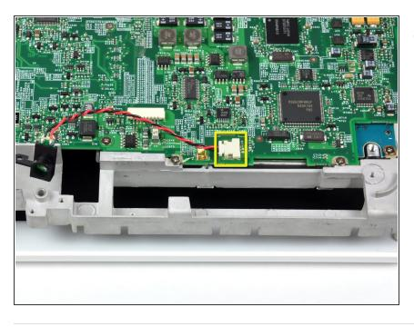
Turn the computer over and disconnect the sleep light from the logic board, removing tape as necessary.
