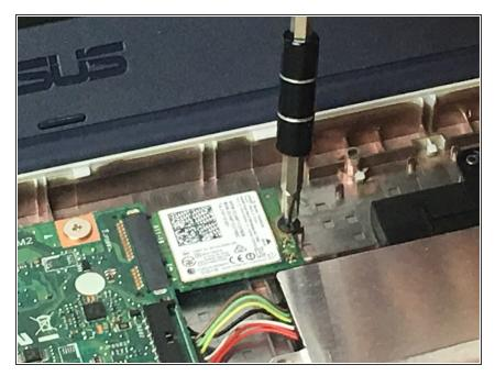
• Unscrew the single 4 mm Phillips #1 screw pinning the wireless card in place.
