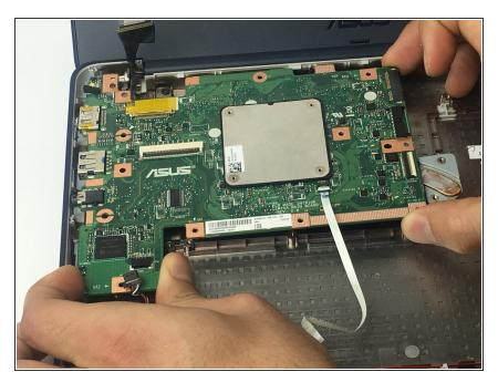
• Lift the motherboard up and out of the chassis.
