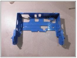
Clean all surfaces of the blue housing with cleaning solution, paper towels, and cotton swabs. Use a pick to clean the debris out of tight spaces.
