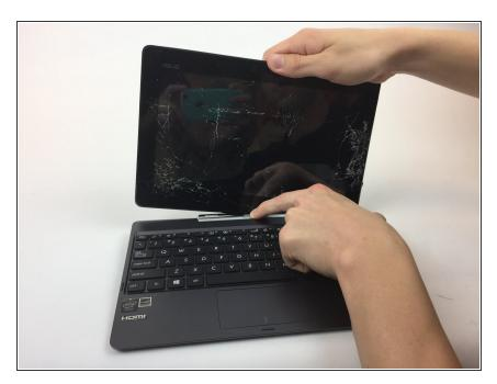
Detach the keyboard from the screen by depressing the silver button on the hinge and pulling upwards on the tablet.
