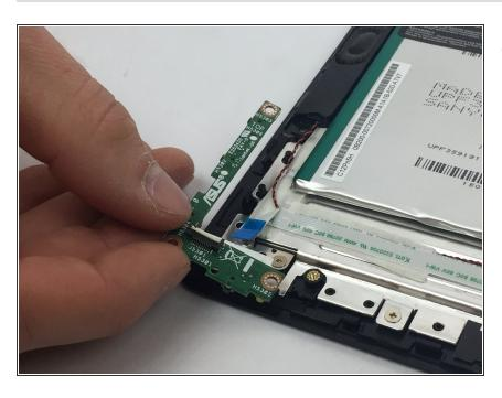
Lift the button module up and out of the device.
