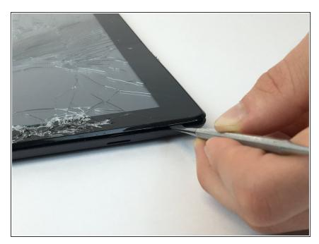
Insert the spudger behind the plastic backing of the tablet and then slide the spudger around the outside of the tablet, carefully releasing all internal clips.
