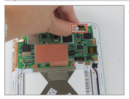
Flip the latch and pull the ribbon cable to disconnect the ZIF connector.
