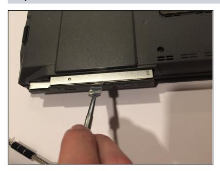
Once the disk-drive has been unlatched from its slot, pull it gently from the laptop case.
