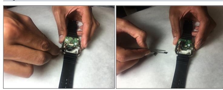
Using tweezers, remove the speaker and move off to the side.
