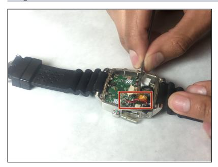
With a pair of tweezers, carefully remove the ribbon strip connection.
