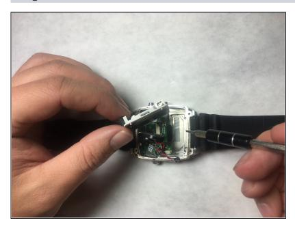
Remove final connection to accelerometer. The LED screen is now separated from the device.
