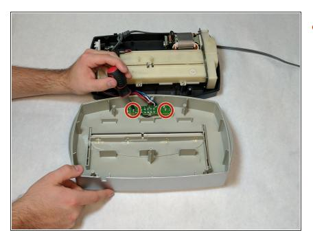
Unscrew both of the screws from the circuit board of the switch. Lift the circuit board away from the device.
