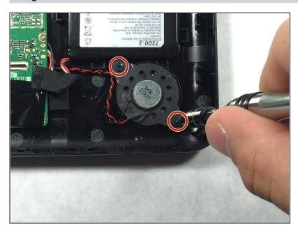
Unscrew the two 5mm screws using a Phillips #000 screwdriver.
