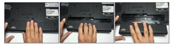
• While continuing to hold the left clasp of the battery panel in place, slide out the old battery by pulling it towards you.
