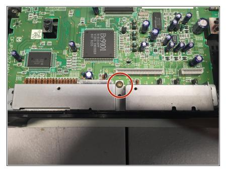
Remove the #1 Phillips Screw from back port cover, and then remove the cover.
