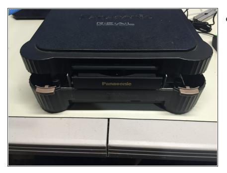
Remove the top portion of the case to expose the internal components.
