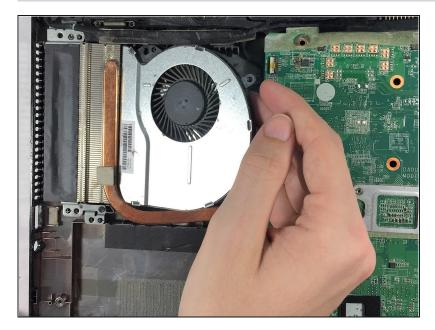
Remove the fan by pulling upward and to the right.
