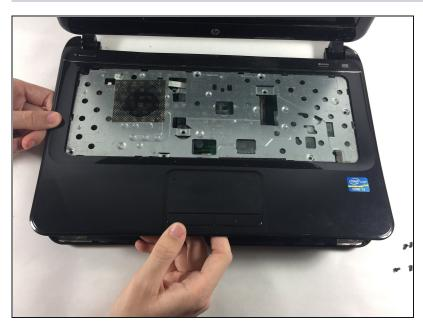
Lift upwards to remove the palm rest.
