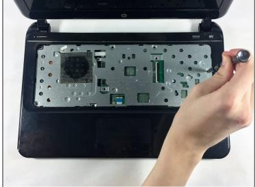
Unscrew the 10 6.0 mm screws under the keyboard housing with a Philips #0 head screwdriver.
