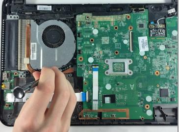
• Unscrew the 3 6.0 mm screws holding the fan with a Phillips #0 head screwdriver.
