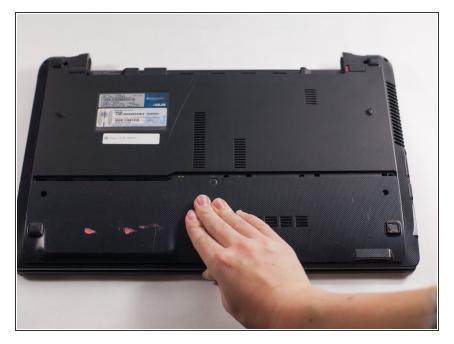
Pull down and lift up on the back panel to remove it.
