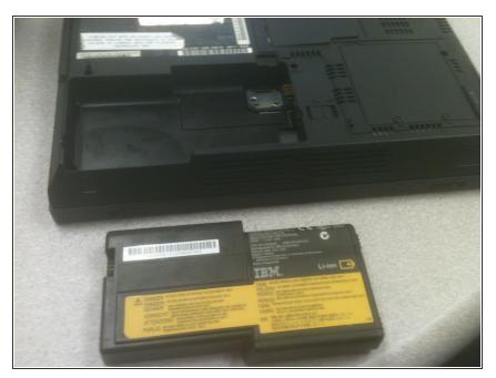
• Remove the battery from the laptop and place it to the side.
