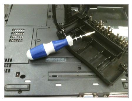
• Use a screwdriver to remove the screws located at the bottom of the laptop, covering the battery pack.
