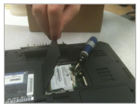
• Loosen the screw covering the Wi-Fi card panel.
