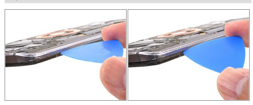
• Insert an opening pick along the frame seam and twist slightly to release the midframe from the phone.
