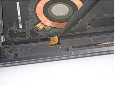
Use the point of a spudger to pry up and disconnect the wireless charging coil connector.
