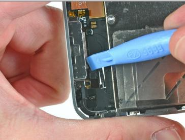
• Use the edge of a plastic opening tool to flip up the retaining flap on the home button ribbon cable.
