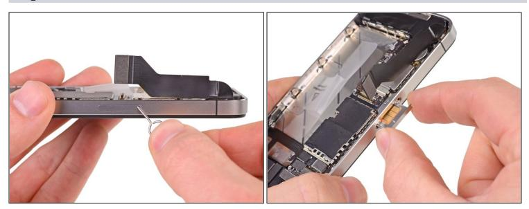
• Use a SIM eject tool or a paperclip to eject the SIM and its tray.
