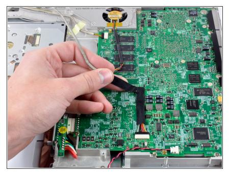
Lift the DC-In cable from the adhesive attaching it to the logic board.
