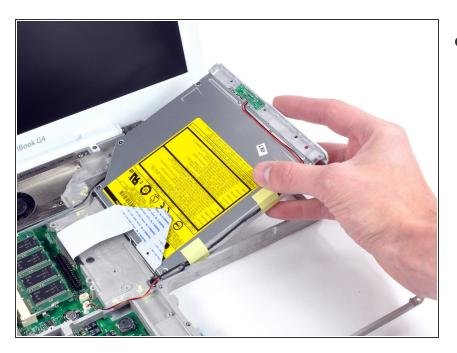
Lift the optical drive from the metal framework.
