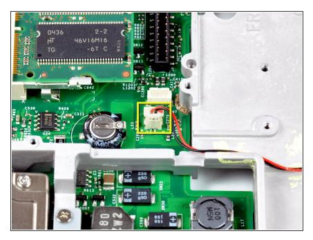
Disconnect the Reed Switch board connector from the logic board.
