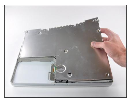
Lift the bottom shield off.
