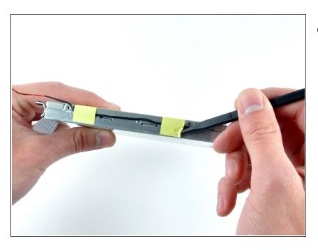
Remove the tape securing the reed switch cable to the optical drive.
