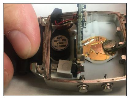
• Use a spudger to lift the battery from the back case.
