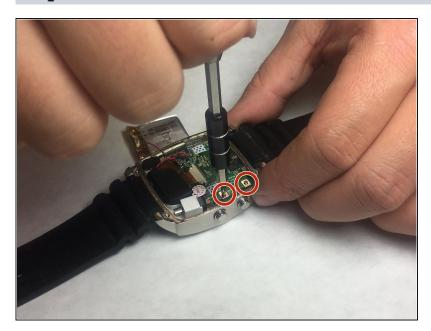
Use PH00 screw driver to remove two 2.4mm Phillips head screws.
