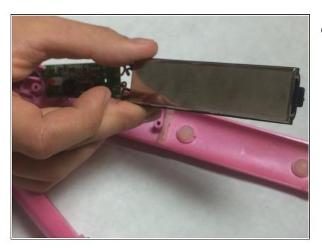
Lift heating plate and circuit assembly away from flat iron case and flip it over.
