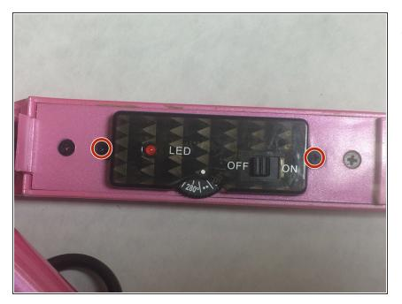
Use the JIS #0 screwdriver to remove the two 3.5mm "J0" screws that attach the control assembly cover to the flat iron base.
