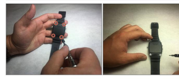
Unscrew the four 3.4 mm flat head screws
