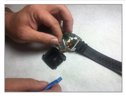
Desolder the battery connections from the motherboard. Learn how to solder components <u>here!</u>
